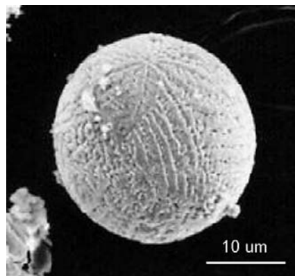
Fe-partikel i flyveaske. (Foto: Microbeam Tech- nologies Inc., North Dakota, USA)
