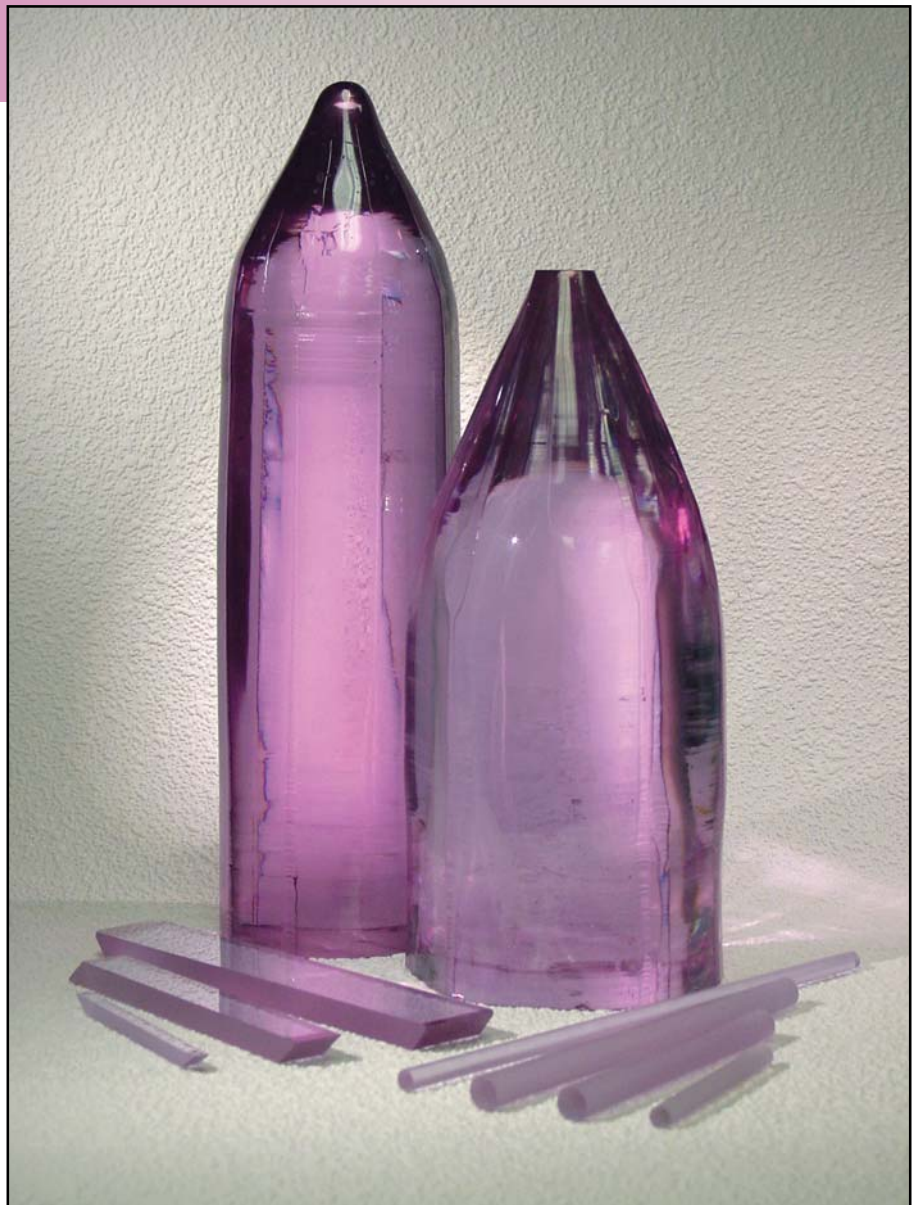
\text{Nd}^{3+} :YAG krystalbouler (de to store krystaller) og færdigpolerede laserkrystaller. (Fotos venligst udlånt af Northrop Grumman Directed Energy Systems – SYNOPTICS via www.st.northropgrumman.com/synoptics )
